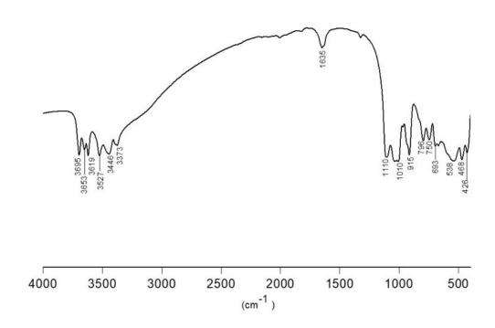
Figure 2. FTIR spectra of bauxite residue sample.
