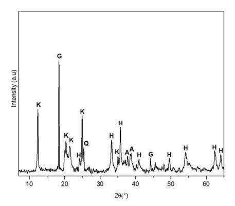
Figure 1. XRD of bauxite residue sample showing kaolinite (K), gibbsite (G), hematite (H), quartz (Q) and anatase (A).
