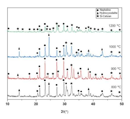
Fig. 5: X-ray diffraction patterns of Sr-exchanged zeolite heated at various temperatures for 1 h.
