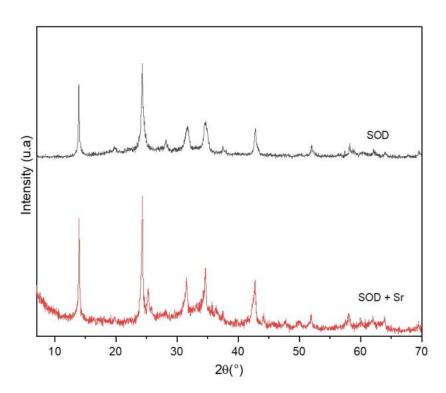
Fig. 4: XRD of Sr-exchanged zeolite hydroxysodalite (red line, SOD + Sr) and zeolite hydroxysodalite (black line, SOD).
