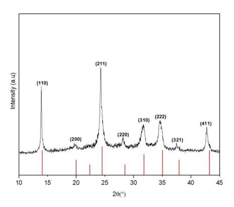
Figure 3. XRD of hydroxysodalite zeolite synthetized from bauxite residue and NaOH.
